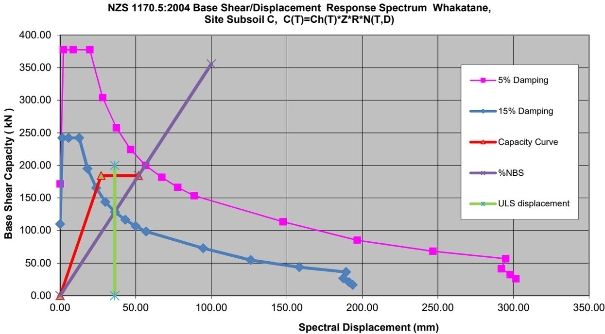
Figure 5 – ULS displacement for IL2
